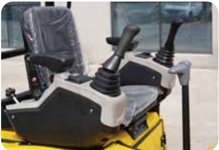
Hydraulic pilot operation
