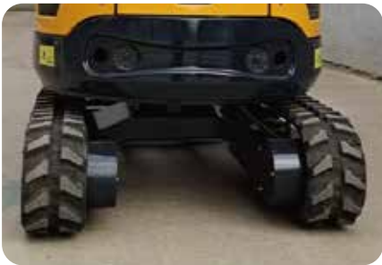
Tailless fuselage, more flexible steering
