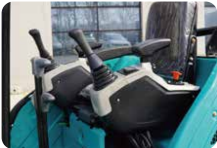
Hydraulic pilot operation
