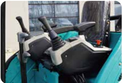
Hydraulic pilot operation
