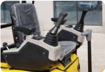
Hydraulic pilot operation
